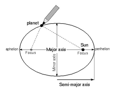
Drawing an **ellipse**: loop string around thumb tacks at each **focus** and stretch string tight with a pencil while moving the pencil around the tacks. The Sun is at one focus.
